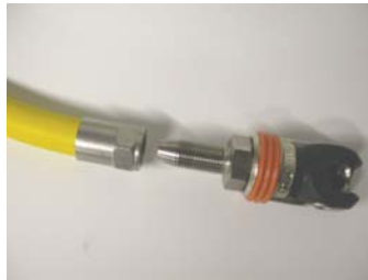
2. Thread coupler into compression fitting.
