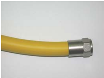
1. Insert hose into compression fitting
