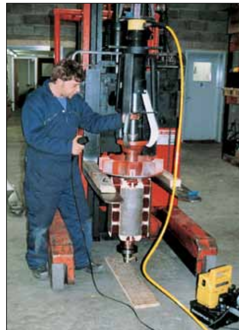
▲ EPHR-116 used to remove electric motor pulleys. Puller is positioned using the Lift Plate.
