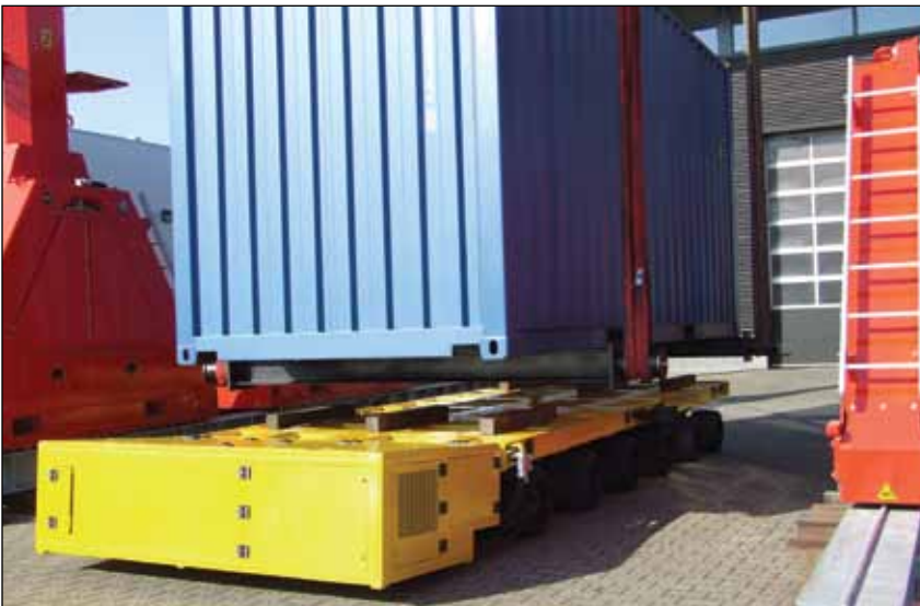
◀ A SPMU used to transport a cargo container in a confined area.
