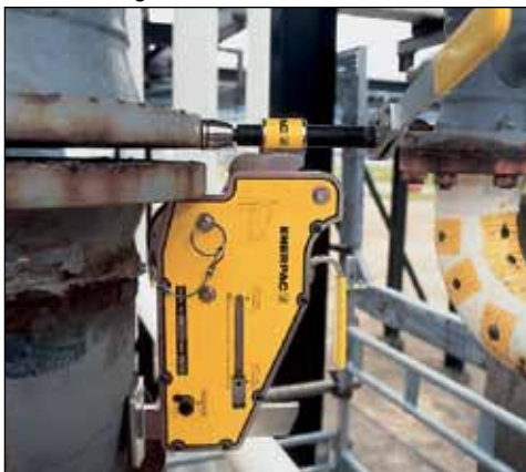
▼ The Enerpac ATM-3 used to align a large ANSI flange.
