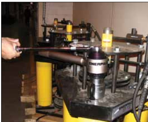
◀ Enerpac Reaction Bar Torque Multiplier E393 used to manually torque bolts up to 3,200 ft-lbs.
