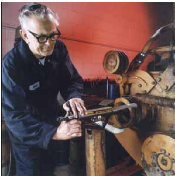
◀ Positioning an EP-104, 3-jaw puller on the accessory drive of a diesel engine.
