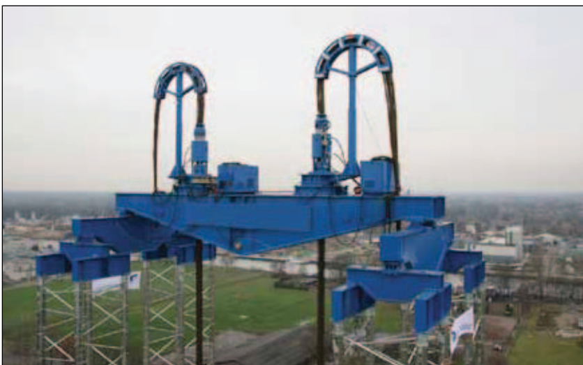
◀ HSL-Series Strand Jack used for heavy lifting market.
