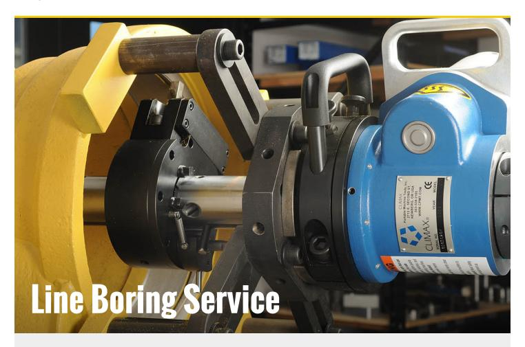
Line boring allows for repair of damaged, out-of-specification pin fits, bushing inserts or barrels at a fraction of the cost of equipment or parts replacement.
