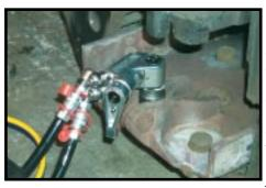
Rail car shock mounting bolts require fast & accurate torquing for change out & maintenance. This rail car maintenance shop relies on a Simplex torque wrench to quickly & easily torque bolts to demanding railroad specifications. "The compact size fits where other wrenches would not & provides more than enough power to do the job right."
