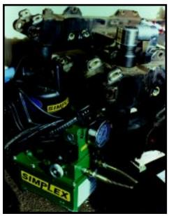
When roller coasters at a popular theme park needed maintenance, park engineers called on Simplex for solutions. Assembly of a critical drive shaft required precision torquing and minimal down time. Simplex power units and square drive wrenches filled the park's needs, saving significant cost and down time.
