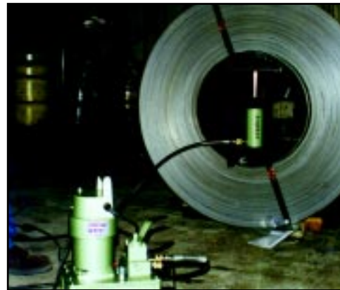
Large steel coils that were damaged in handling are reshaped using a Simplex R256 cylinder and PE70 Series pump.
