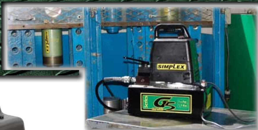
The G5 power pump coupled with a 50 ton Simplex cylinder are used daily to position bearings in the assembly processing section of the plant.
