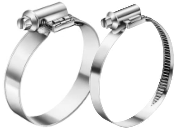
The embossed, non-perforated band on OETIKER worm drive clamps prevents radial damage to the hose. OETIKER worm drive clamps conform to all requirements of DIN 3017, in particular to the required installation torque.
