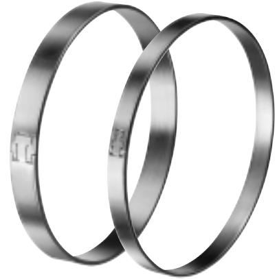
OETIKER Multi Crimp Rings are made from band steel, have a T-lock and their low profile makes them particularly suitable for large rotating parts as they have no protruding parts to obstruct the space surrounding the hose.
