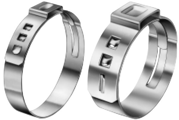
The term "Stepless" refers to the absence of steps or gaps on the inner circumference of the clamp. The ingenious stepless design provides uniform compression and a 360° seal.
