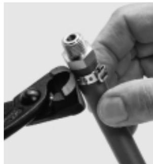
To release stepless clamps, grip end of band with pincers and pull off.
