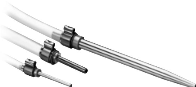
OETIKER 1-ear clamps with Insert are ideal for demanding hose or tubing clamping applications involving soft or hard rubber or plastic materials. The insert bridges the gap below the clamp ear and its curled edge prevents cutting or other damage to the hose.
