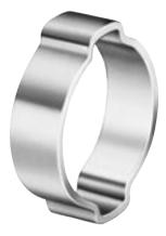
The 2-ear clamps have a larger clamp range than the 1-ear clamps. The closed "ear" geometry provides an inherent retained load and a spring action in the clamp, permitting expansion and contraction during thermocycling or vibrating conditions. For proper installation and seal, both "ears" must be crimped closed.
