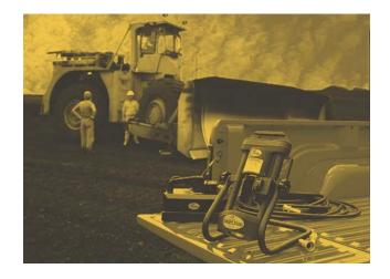
That's because hoses, couplings, assembly equipment and crimping tolerances vary from one manufacturer to another, and they're not interchangeable. When components from different manufacturers are mixed together, coupling retention can be adversely affected. Mixing components can not only cause unnecessary downtime, it can result in personal injury as well. In addition, the thread or flange ends of couplings must be properly matched to their mating components to create leak-proof connections.
