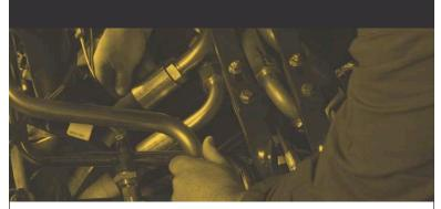
Periodic hose assembly inspections can prevent unwanted and unexpected assembly failures. During normal operations, be aware of how the equipment sounds, feels, etc. Be sure to check any noticeable abnormalities.
