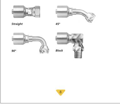
Hose ends and thread ends are measured by industry standard dash sizes. The hose end dash size refers to the inside diameter in 1/16" (except for PolarSeal® hose, SAE100R5 and SAE100R14 which are based on tube O.D. and are one size smaller than the dash size implies) i.e. – 8C5C hose is actually 13/32" I.D.
