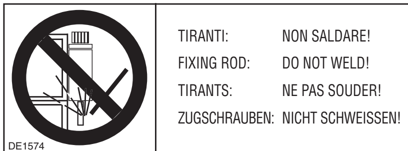
DE 1574 Do not weld the fixing rods
