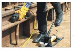
Easily removing rusty nuts during railroad construction is just one of many application examples for the Enerpac Nut Cutters.
