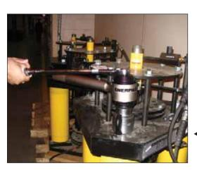
■ Enerpac Reaction Bar Torque Multiplier E393 used to manually torque bolts up to 3,200 ft-lbs.
