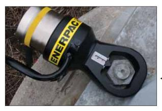
Heavily corroded and weathered nuts are quickly split and removed using an NS-Series Nut Splitter.
