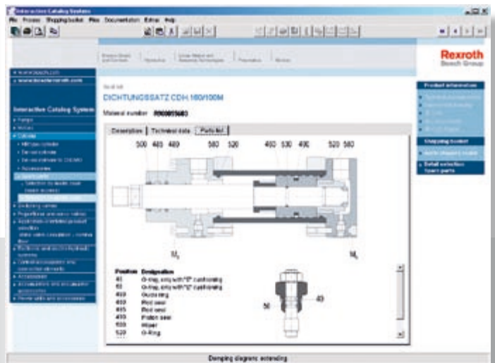
Spare parts drawing with individual parts and material number for the associated sealing kit
