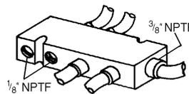
Use the #20 die cast aluminum manifold to simplify piping and cut down on plumbing time. A 3/8" NPTF inlet port provides a common air source for up to eight 1/8" NPTF outlets.
