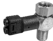
Port mounted SCS valves emit an air signal when the cylinder rod has stopped even if the piston has not contacted the end cap. SCS valves are ideal for use in situations where the full cylinder stroke is not used. SCS valves are available in 1/8", 1/4", 1/2" pipe sizes. See pg. 57.
