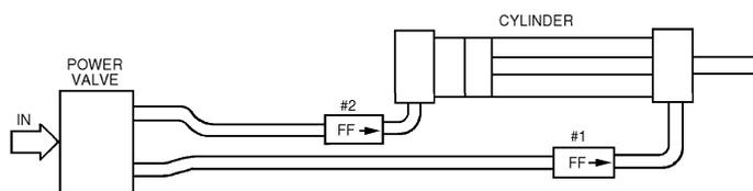
In this circuit, flow control #1 controls the outward movement of the cylinder rod and flow control #2 controls the return speed.
