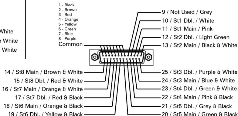
NOTE: All Commons are connected internally on both the 4 and 8 Station Manifolds.
