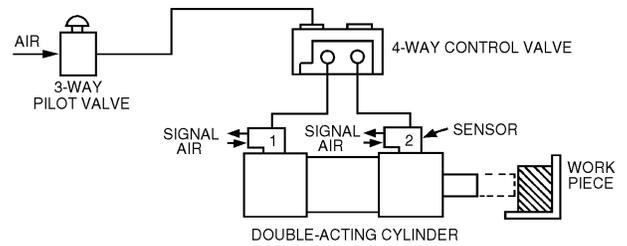
In this sample circuit, sensor #1 provides an air signal when the cylinder rod is retracted. When the four-way control valve shifts, air flows to the cylinder, which extends. This causes sensor #1 to shut off. The cylinder rod stops when it reaches the work piece or end of stroke, causing sensor #2 to emit an air signal. This air signal may be used to actuate another valve or for sequencing operations.
