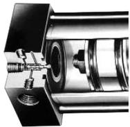
A miniature 3-way valve built into the cylinder head is actuated by the cylinder piston as it reaches the end of its stroke. Once contacted, the 3-way Inter-Pilot® valve emits an air signal. In this manner, sequencing is achieved without external limit switches and electric wiring.
