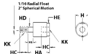
DMC-1 Forged Rod Clevis w/Pin
