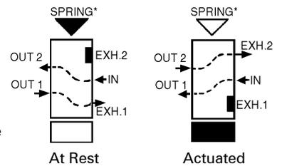
\*On double solenoid or double air piloted models, the second actuator replaces the spring.
