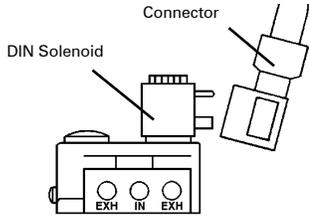
A DIN connector (ordered separately) quickly attaches to the solenoid's prongs and is secured by a single screw.
