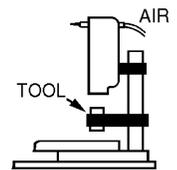
The air hammer's impact force may be adjusted from a few ounces to 4,500 lbs. by raising or lowering the air hammer, adjusting the air trip needle valve, or adjusting the air pressure. The air trip mechanism releases the hammer head when the air in the chamber reaches a pre-set level. The hammer head accelerates to the end of its stroke, with a longer stroke (6" maximum) creating greater velocity and greater impact.
