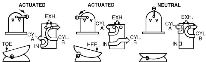
Note: In neutral, cylinder ports are dumped to atmosphere.
