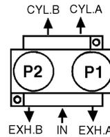
Single-actuated spring return models, including hand lever and foot pedal, have the inlet and Cyl. B ports connected when unactuated. On all double-actuated models, except N2-PB and N2-DB, signals at P1 cause output at Cyl. A and signals at P2 cause output at Cyl. B. On N2-PB and N2-DB models, the reverse occurs.
