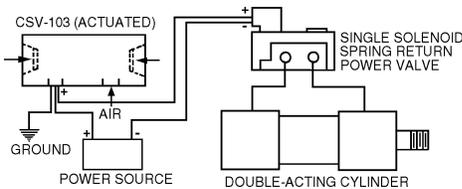
Converts an air signal into an electrical signal for actuating solenoid valves or other electrical devices. Concurrent actuation of the recessed buttons produces an electrical output. Releasing one or both buttons stops the output. The CSV-103 will not recycle until both triggers are released and again actuated concurrently. Internal switch rated at 15 amps, 480 VAC. Includes lead wire and receptacle.
