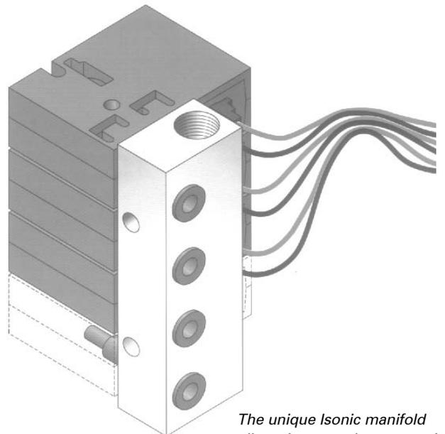
The unique Isonic manifold allows instant valve connection and removal, without the aid of a tool.
