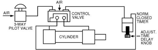
In this circuit, the 3-way valve is actuated and air is sent to the control valve. The control valve shifts, sending air through port A to the cylinder, which extends. Air also flows to the timer where it begins to time to the pre-setting. Once reached, the timer opens, allowing the air to flow through to the control valve's other pilot port, shifting the valve back. Air flows through port B, retracting the cylinder.
