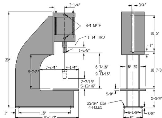
For non-standard double-acting service with strokes up to 6", use pages 34-35 to design a 6" bore cylinder for use with this stand.
