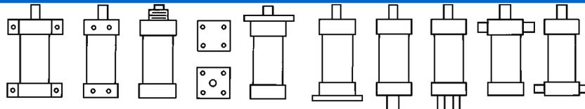
Foot    Bottom    Flush    Nose    Frt/Rear    Front    Flange    Rear    Pivot    Clevis    Trunnion    Trunnion
