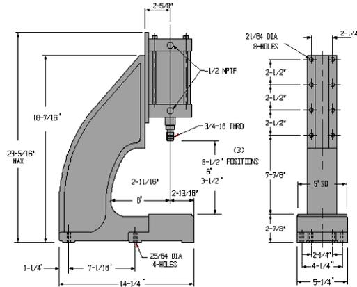
For non-standard double-acting service with strokes up to 4", use pages 34-35 to create a 4" bore cylinder for use with this stand. The PL-400 cylinder-to-stand adapter plate will be required.
