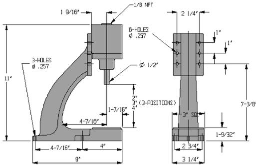
This press combines the AP-42M press stand with a Mead H-42 single-acting cylinder (2 1/4" bore, 2" stroke). Cylinder details are on page 51.
