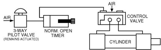
When the 3-way valve is actuated, air flows through the NO timer to the control valve. The 3-way valve remains actuated. The control valve shifts, sending air through port A to the cylinder, which extends. At the same time, the timer begins to time to the pre-setting. Once reached, the timer closes, blocking off the air flow to the control valve, which springs back. Air flows through port B, retracting the cylinder.
