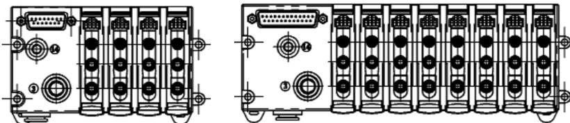
NOTE: Valve 1 is located nearest to Serial Connector, Common Pins are connected internally.
