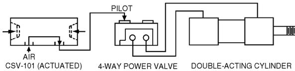
Will actuate any 3 or 4-way air piloted, spring return power valve or small single-acting cylinders. ( $C_v = 0.11$ )
