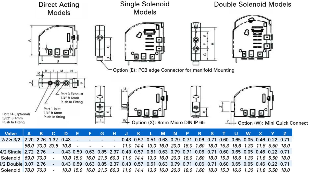
Note: Sizes are in inches first, millimeters second (italicized).
