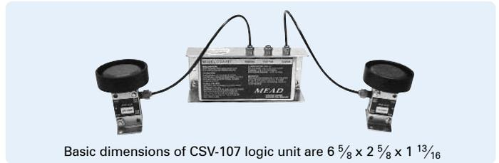
Basic dimensions of CSV-107 logic unit are  $6 \frac{5}{8} \times 2 \frac{5}{8} \times 1 \frac{13}{16}$
