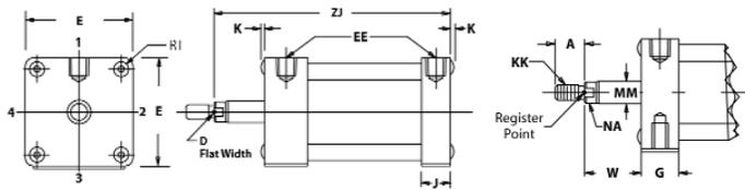
**NOTE:** DM1 Cylinders are constructed with sleeve nuts; use RT, K does not exist. DM2 use K; RT does not exist.
