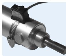
Hall Effect & Reed switches can sense rod position anywhere within the stroke. A stainless steel clamp facilitates mounting at any location along the cylinder tube. Switches may be used singly or in multiples and positioned at any point around the cylinder tube. The cylinder must have a magnetic piston. For technical information see pg. 33.
