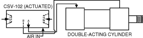
Complete power package containing a 4-way power valve ( $C_v = 1.00$ ) for direct actuation of single-acting or double acting air cylinders. Actuation sends a sustained air flow to one cylinder port. Releasing one or both buttons shifts the flow to the other cylinder port. Built-in mufflers reduce sound levels. Quick-connect fittings included.
