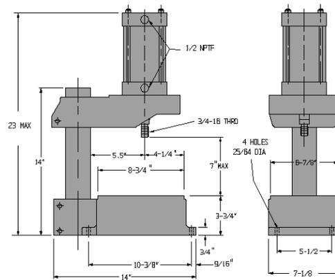
For other stroke lengths, heavy-duty or other options, use pgs. 34-35 to create any 4" bore cylinder for use with this press stand.
