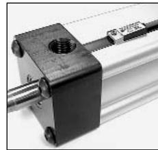
Hall Effect and Reed Switches allow the cylinder user to sense rod position anywhere within the stroke. Switches are available for both models. For the DM1 series the switch attaches to any of the four tie-rods. For the DM2 series, a dovetail slot runs along the cylinder tube to facilitate fast and accurate position setting.
