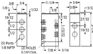
Note: Envelope dimensions of valves with actuators are shown in the chart on the right.
