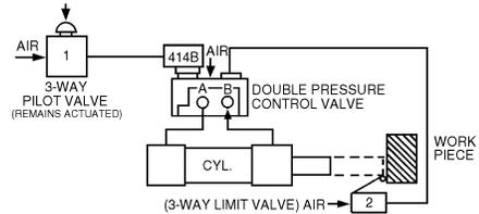
When actuated, the 3-way valve sends a signal to 414B, which emits a signal to the control valve. The 3-way valve remains actuated. The valve shifts, allowing air to flow through port A, extending the cylinder. 414B senses the back pressure caused by the shifted valve, closes, and exhausts. Since the signal from valve #1 is blocked by the closed 414B, valve #2 (when actuated) shifts the control valve back. Air flows through port B, retracting the cylinder.
