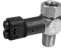
Port mounted SCS valves emit an air signal when the cylinder rod has stopped even if the piston has not contacted the end cap. SCS valves are ideal for use in situations where the full cylinder stroke is not used. See pg. 57.
