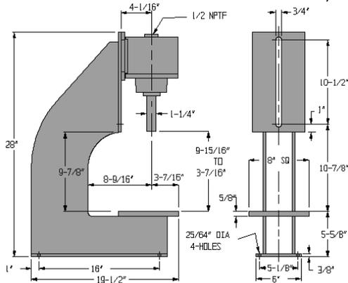
This press combines the AP-600M stand with Mead's #6040303 (H-283 with 3" longer ram, p. 51) single-acting cylinder (6" bore, 3" stroke). A PL-600 cylinder-to-stand adapter plate is required to mount this cylinder.
