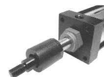
Rod couplers simplify cylinder alignment problems by compensating for 2° angular error and 1/16" lateral misalignment on both extension and retraction strokes. Greater reliability is achieved by reducing cylinder and component wear. All components are heat treated for wear and corrosion resistance.
