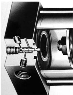
Mead's Inter-Pilot® is a miniature 3-way valve built in the cylinder head. Actuated by the cylinder's piston as it reaches the end of its stroke, the valve emits an air signal. Thus, sequencing is achieved without external limit switches and electric wiring.
