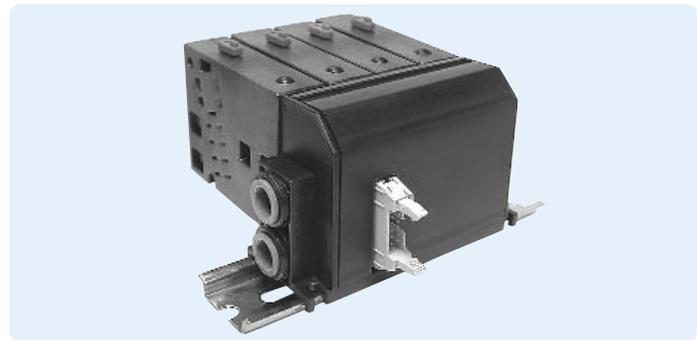
Pre-wired manifolds are supplied with a protective cover. The cover snaps easily into place to protect the wiring and circuit board. It is easily removed for servicing or replacing a valve.
