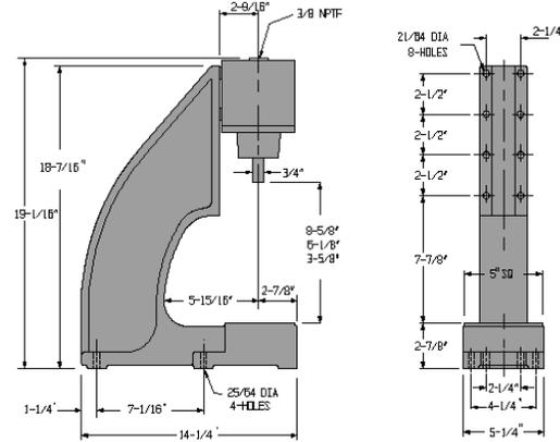
This press combines the AP-400M press stand with a Mead H-122 single-acting cylinder (4" bore, 2 5/8" stroke). Cylinder details are on page 51.
