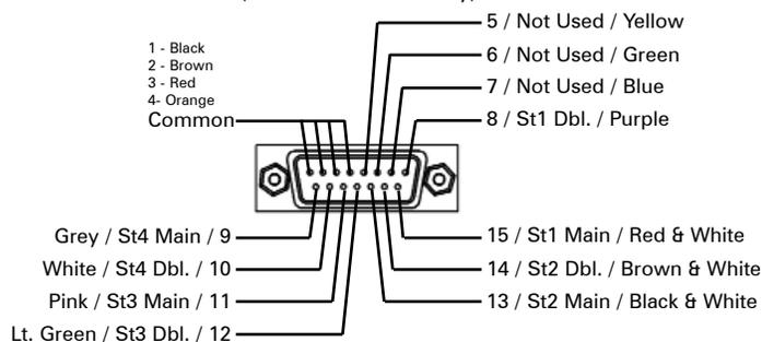
Detailed Explanation: St1 Main = Station 1, Main connection (Used for all valves installed here).
