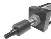
Rod couplers simplify cylinder alignment problems by compensating for 2° angular error and 1/16" lateral misalignment on both extension and retraction strokes. Greater reliability is achieved by reducing cylinder and component wear. All components are heat treated for wear and corrosion resistance.
