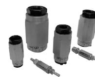
**Dyla-Trol®** - For unprecedented smoothness in cylinder speed control, use Mead's Dyla-Trol® valves with a perfectly tapering flow. Where needle type flow controls generate turbulence as they close, Dyla-Trol maintains an even 360 laminar flow regardless of the setting. Pg. 59.
