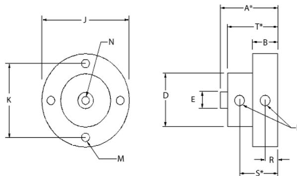
NOTE: 3/4" - 2" Bore Models have (2) Mounting Holes. See Dimension M.
