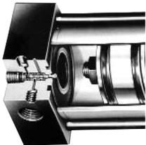
A miniature 3-way valve built into the cylinder head is actuated by the cylinder piston as it reaches the end of its stroke. Once contacted, the 3-way Inter-Pilot® valve emits an air signal. In this manner, sequencing is achieved without external limit switches and electric wiring.
