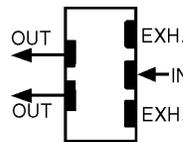
Capsula valves are 4-way, 5 ported directional control valves. This means that they have one inlet, 2 pressure outputs, and 2 exhaust ports. Dual exhausts facilitate individual flow control of each output port and allow dual pressure and diverter hooksup.
