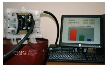
Why Count Cycles? Counting the number of cycles provides a method of measuring how much fluid is being transferred through the pump. Every time a cycle is completed, an impulse is sent from the cycle count valve. This impulse can be interpreted by a data acquisition center for automated input to a PC, PLC, relay or switch. The control device can then regulate a valve on the air line or fluid discharge line based on a measured number of cycles.
